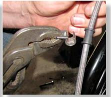
Drill out the factory p-clamps until they snap off, then remove the clamps from the upper arm.
