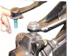
Disconnect the **tie rod** from the knuckle. (**18mm**)
