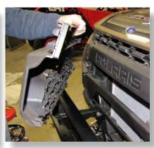
Remove the front grill insert to gain access to the sway bar.
