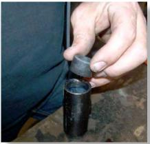
You will need to reuse your factory pivot caps, bushings, sleeves, and ball joints. Make sure that you inspect your bushings and ball joints for wear. Replace as needed.
