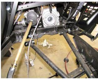
Remove the Upper and Lower arms by removing the bolts from the frame. (18mm) Then remove the stock axle. KEEP ALL FACTORY HARDWARE.
