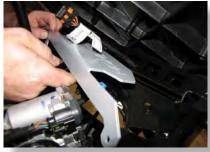
Disconnect and unclip the wire. Slide the logo plate (61Z) between the frame bracket and the bed.
