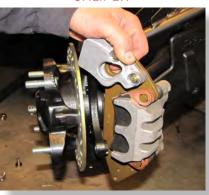
Disconnect the **brake lines** from arms and frame. Remove the **(2) brake caliper mounting bolts (15mm) Do NOT disconnect lines from caliper.** Set brake caliper aside.
