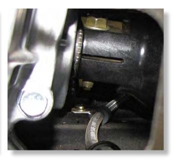
Run the slack out where the brake line runs under the rear differential. Make sure the line is still running through the two clamps attached to the bottom and clear from contacting the rear drive shaft.
