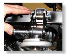
Connect the top of the shock to the lift brackets using one (10x65mm bolt) and (10mm lock nut).
