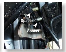
Insert a spacer (CCC) on each of the bolts. Now place the front long lift bracket to the inside of the inner shock mount tab. Push the two bolts all the way through and loosely fasten it with (two 10mm lock nuts).
