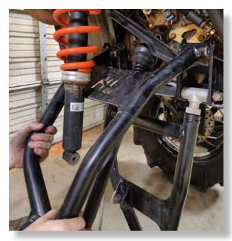
Install the new **APEXX upper control arm** to the frame, using the factory hardware. **DO NOT FORGET WASHERS.**
