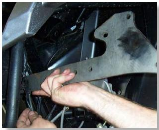
Run the long front lift bracket (72Y) behind the wires and along the frame support bars to the other side. You will insert the bracket into the center of the two shock mount tabs on both sides of the UTV.
