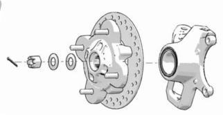
Reattach the rotor to the knuckle assembly.
