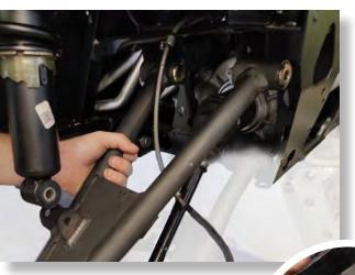
Using factory hardware, connect the new upper arm to the frame, then at the pinch bolt on the knuckle.
