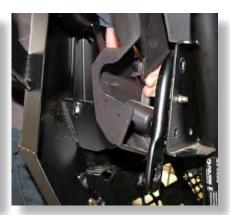
Slide the sway bar out and through the other end, then reconnect the front grill insert.
