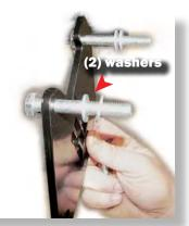
Place one rear lift bracket (86N) to the outside of the rear shock mount. It needs to be on the side that faces the front of the UTV.
