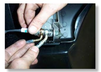
Disconnect the banjo bolt and brake lines from the master cylinder.
