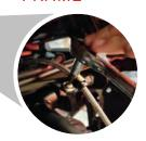
Secure brake line to frame with a p-clamp, using factory hardware.
