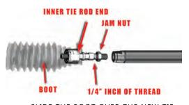
SLIDE THE BOOT OVER THE NEW TIE ROD. NOW INSTALL THE TIE ROD END TO THE RACK AND ONCE THE NEW TIE ROD IS INSTALLED SLIDE THE BOOT OVER THE TIE ROD END AND SECURE WITH ZIPTIES.
