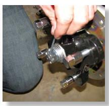
Place the rotor onto the hub and axle assembly. Fasten the rotor using the axle washers, castle nut, and cotter pin provided in the kit.
