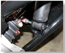
Use the 10mm x 65mm bolt to connect the lower portion of the shock to the control arm.
