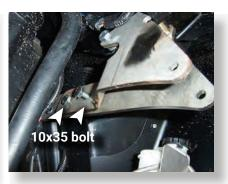
Use (two 10mm x 35mm bolts) to secure the short front lift brackets to the long front lift bracket.
