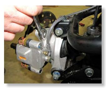
**Disconnect the caliper** bolts from the hub assembly, leave the brake line attached to the caliper (15mm). Set brake caliper aside. **KEEP FACTORY HARDWARE**.
