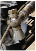
Use a 1/2" drill bit to drill out the factory hole where the original tie rod connected. Slide the (5/8-18"x5" bolt) through the alignment bushing the heim joint, and the riser cone, then insert through the knuckle assembly and fasten with the 5/8-18" lock nut with a washer.
