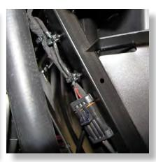
First, unclip the wires from around the upper shock mount tabs. These can interfere with the installation.
