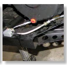
Locate the brake line junction block on the rear driver side or left side of the frame. Disconnect the rear driver side line from the junction block. Connect the new 6" extension (46Y) to the brake line and then to the junction block.
