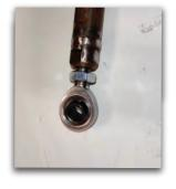
Install the heim joint and jam nut to the opposite end. This will likely need to be adjusted later.
