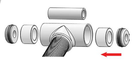
Once the bushing is inserted, use a socket, of the same diameter as the bushing to press it in all the way.
