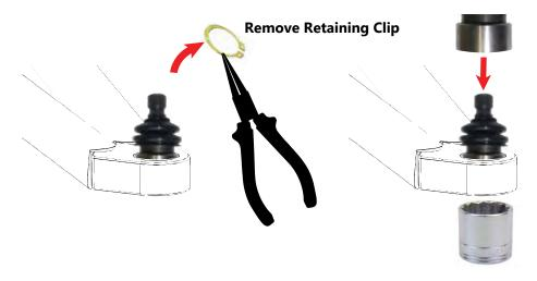
Back the ball joint with a large 36mm socket or something sturdy of similar diameter, then using a press or vice, press the ball joint out of the arm.
