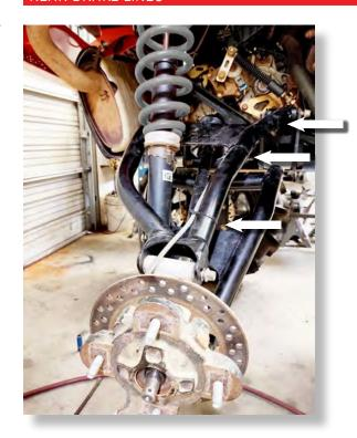
Secure the rear brake line to the front of the upper control arm using 3 (8" zip ties)
