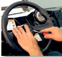
(B) If the steering wheel is not centered, you will need to remove the center cap with a flat head screwdriver to gain access to the steering wheel nut.
