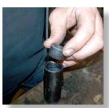
**CAUTION:** There is a stop built into the factory arm that prevents the bushing from pushing out when installed. Because of this, the bushing must be pushed out from the opposite side.
