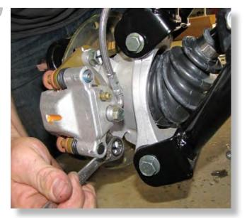
Fasten the calipers to their hubs. (15mm)
