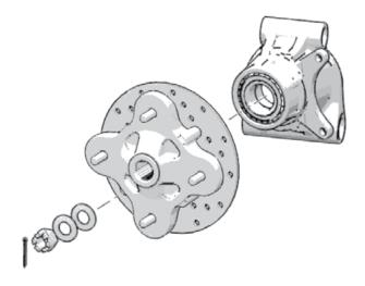
Remove the factory cotter pin and castle nut (27mm) on the rear axles, then remove the brake rotor assembly.
