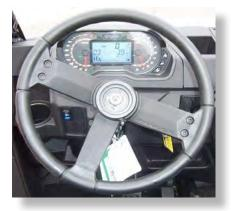
A) When the steering is zeroed, check the steering wheel to make sure that it is properly positioned.
