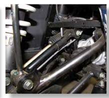
Disconnect the brake line from the caliper and upper control arm. Have a container ready to collect brake fluid.
