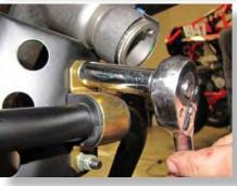
Remove the nuts that secure the sway bar to the sway bar rod. **COMPLETELY REMOVE THE SWAY BAR**, **sway bar connecting brackets**, **and rods from the UTV**. They are not used in conjunction with the big lift kit.
