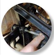
(If installed from the opposite direction, the exhaust will continue to block bolt removal)
