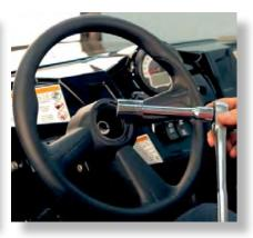
(C) Using a ratchet, turn the steering nut counter clockwise or left. Continue this until the steering wheel locks at full turn, then loosen the nut. Do not remove the nut yet.
