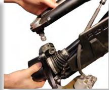
Disconnect the **Upper ball joint** by removing the **bolt** at the knuckle. **(15mm)**
