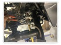
REMOVE CLAMPS AND/OR ANY ZIP TIES HOLDING THE BOOT IN PLACE. NOW, SLIDE THE BOOT DOWN THE TIE ROD.
