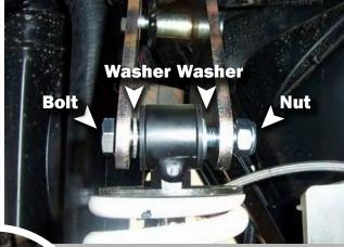
Insert the 10mm x 65mm bolt through the upper shock lift bracket, then slide it through the (2) 10mm washers. Secure it with a 10mm lock nut.
