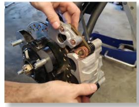
Connect the caliper to the hub assembly.
