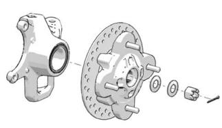
Remove the cotter pin, axle nut, and washers from the hub assembly, then remove the hub. (27mm) KEEP FACTORY HARDWARE.
